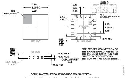
Figure 31. 16-Lead Lead Frame Chip Scale Package [LFCSP] 3 mm × 3 mm Body and 0.75 mm Package Height (CP-16-22) Dimensions shown in millimeters
