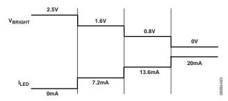
Figure 22. PWM Brightness Control Application Diagram Using a DC Voltage Applied to  $V_{BRIGHT}$
