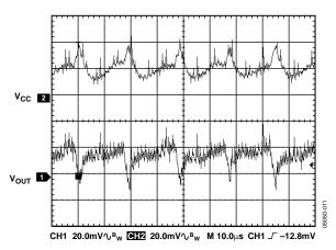
Figure 10. 1.5× Mode Operating Waveforms
