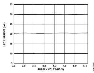
Figure 7. ILED (mA) vs. Supply Voltage (V)
