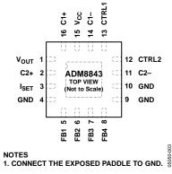
Figure 2. Pin Configuration
