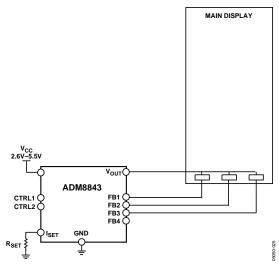
Figure 24. Driving Three White LEDs
