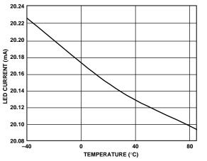
Figure 4.  $I_{LED}$  (mA) Variation over Temperature (°C),  $V_{CC} = 3.6 \text{ V}$
