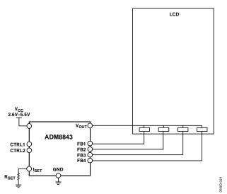
Figure 23. Driving Four White LEDs
