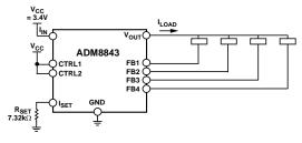
Figure 30. Charge Pump Power Efficiency Diagram, Example 1
