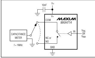
Figure 5. Channel Off/On-Capacitance
