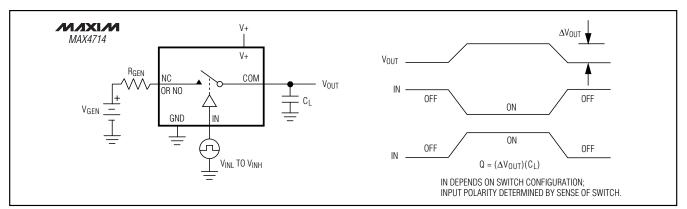
Figure 3. Charge Injection
